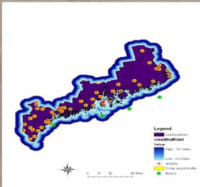
Each buoy location also contains the average wind speed of the location. Using the Kriging function in the geostatistical analyst of ArcGIS I took the average wind speeds of the four known buoy locations and interpolated (calculated) the missing wind speed values
