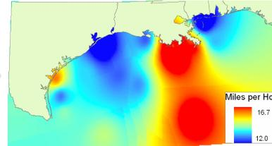
**Figure 3:** Average hypothetical wind speeds from March 5, 2005 through April 20, 2005 in the Gulf of Mexico. Bulls-eye distribution is a result of the IDW calculation process, which assumed maximum wind speed at the buoy and that wind decrease as measurements proceed away from the buoy in any direction.
