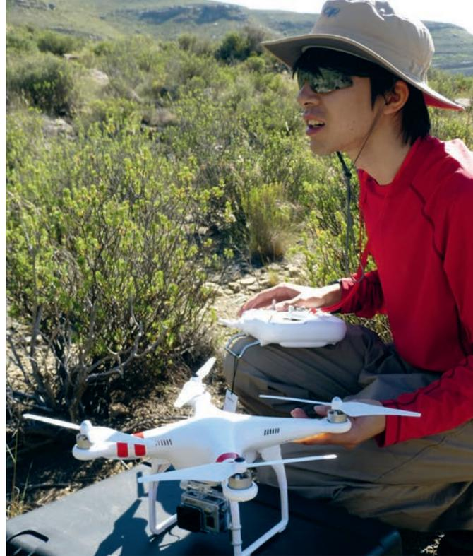
*Tak Sasajima '16 readies the research team's DJI quadcopter for a flight along the mountain's edge to record images of resistant sandstone features. Images from the quadcopter are used to generate three-dimensional models, allowing the team to reconstruct the original river system.*
