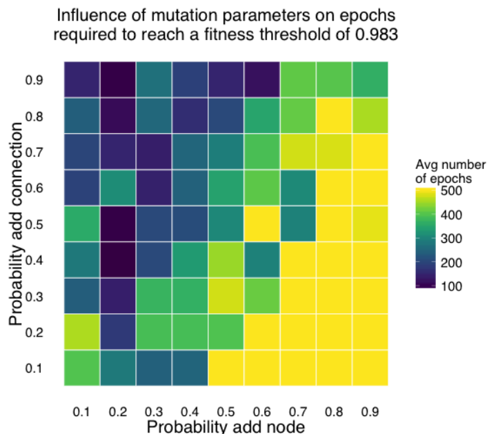
Figure 5: A heat map showing the average number of epochs needed to reach a 1 - MSE threshold of 0.983 as a function of the probability of adding a node and the probability of adding a connection during mutation. It suggests that an optimal combination is found when the probability of adding a node is 0.2 and the probability of adding a connection is 0.4 or 0.5.
