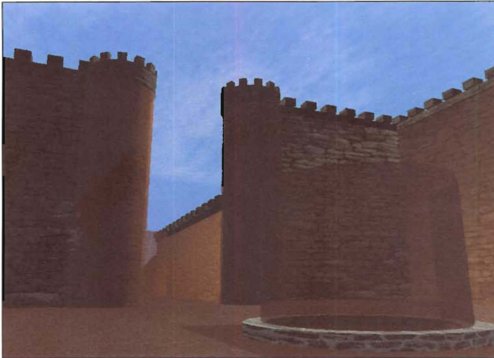
Figure 12.2 This screenshot shows collision boundaries in a translucent red color. Notice the flat polygons on the floor and walls, and the cylindrical boundaries around the turrets and well. Notice with the well that something need not be drawn for a boundary to exist; in the well's case, it is the absence of a floor that requires a boundary, so the viewer cannot fall down the well.
