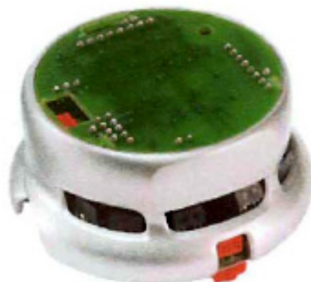
Figure 3.2: Front view of the Khepera robot showing infrared sensors 1 through 5. Photo courtesy of [5].
