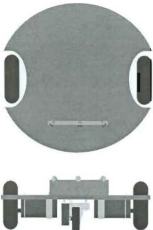
Figure 3.2.7 – Robot base with light sensors
