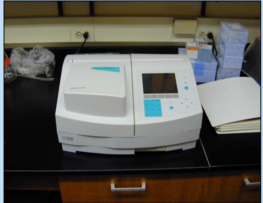
Milton Roy Thermospectronic Aquamate Spectrophotometer used to test phosphorus samples
