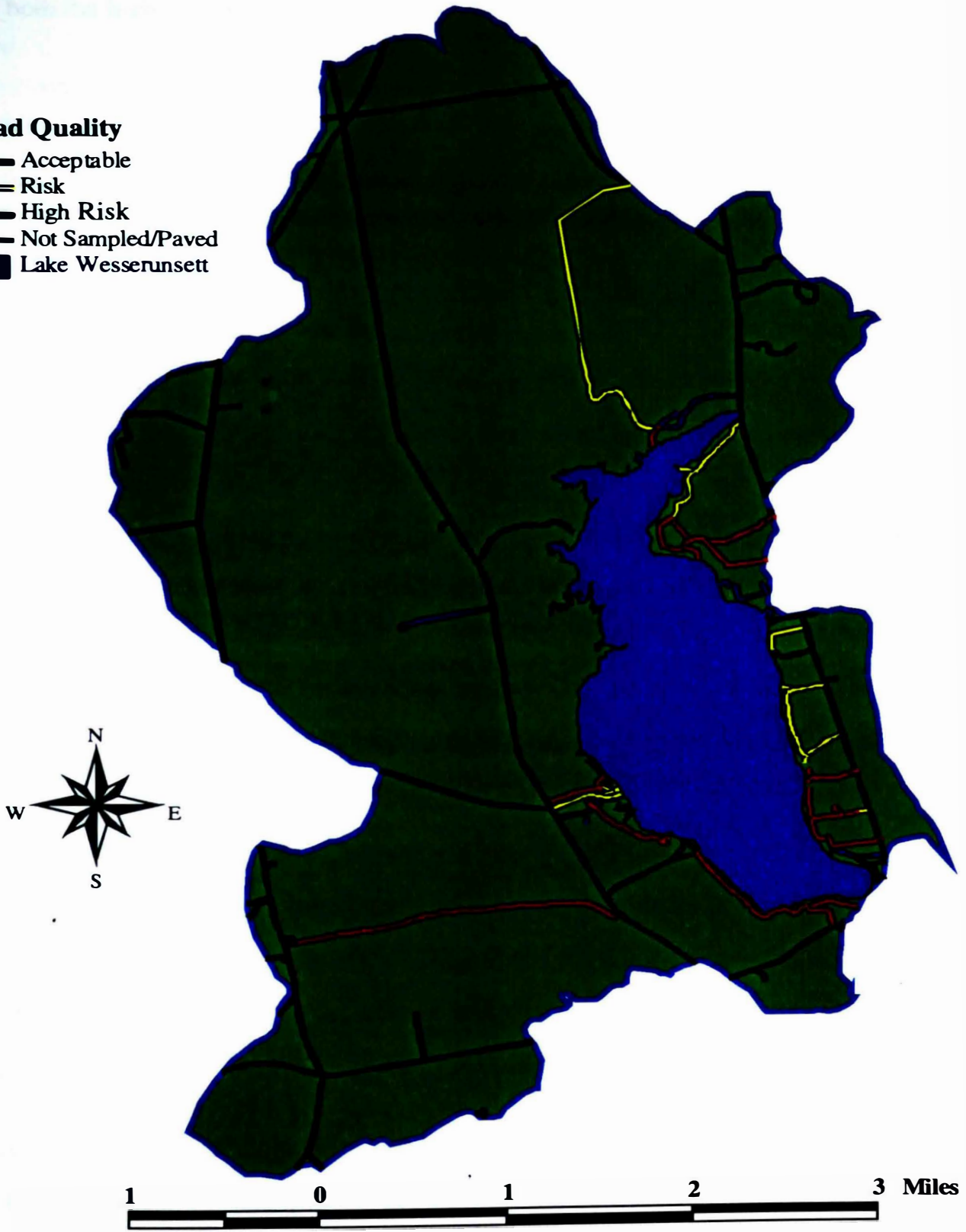
Figure 27. Condition of detailed surveyed roads in the Lake Wesserunsett watershed based on road ranking data from Table 10. High risk roads in close proximity to the lake should receive priority in maintenance to prevent adverse water quality effects.
