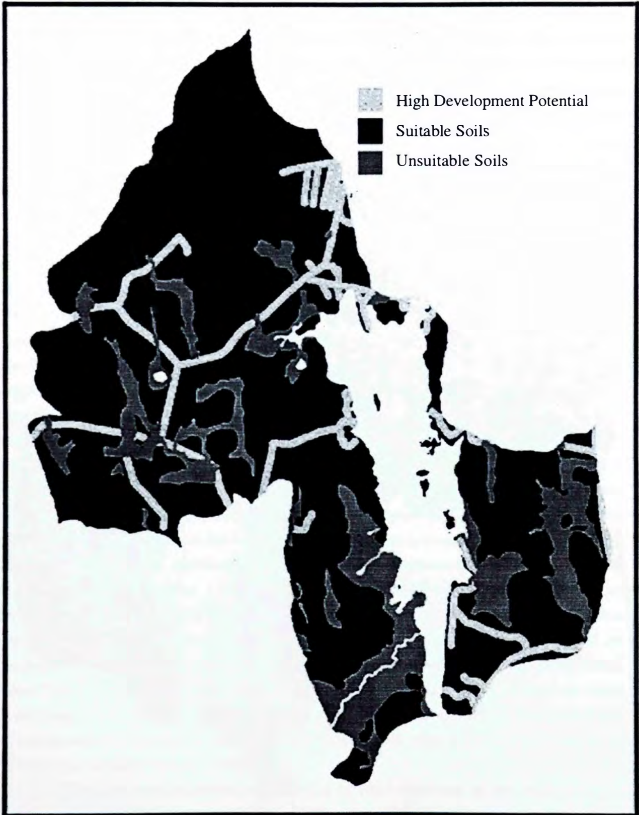
Figure 36. Development projections based on soil suitability and existing roads and power lines. High potential area is a 50m spread around existing roads.
