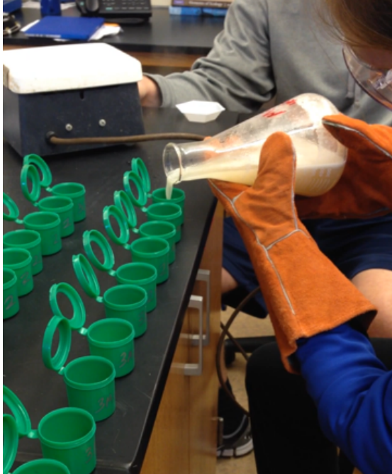
Figure 8.2 Method of pouring hot agar solution into 35mL poly-con cups.
