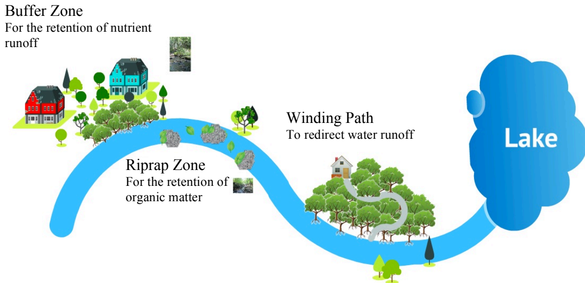
Fig. 8.2. Types of conservation actions that can be implemented on headwater streams.
