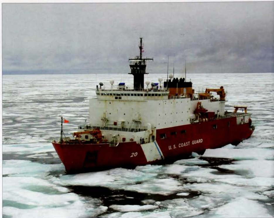
The U.S. Coast Guard icebreaker and research ship Healy, during its Northwest Passage voyage. The ship can ram through ice eight feet thick.
