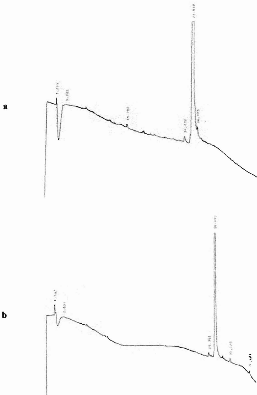
Figure 10: Analytical HPLC traces of purified oligonucleotides. Absorbance (260nm) vs. time (min) for (a) strand 1 and (b) strand 2. Both traces were obtained using linear gradient of NaCl (Table 1a)
