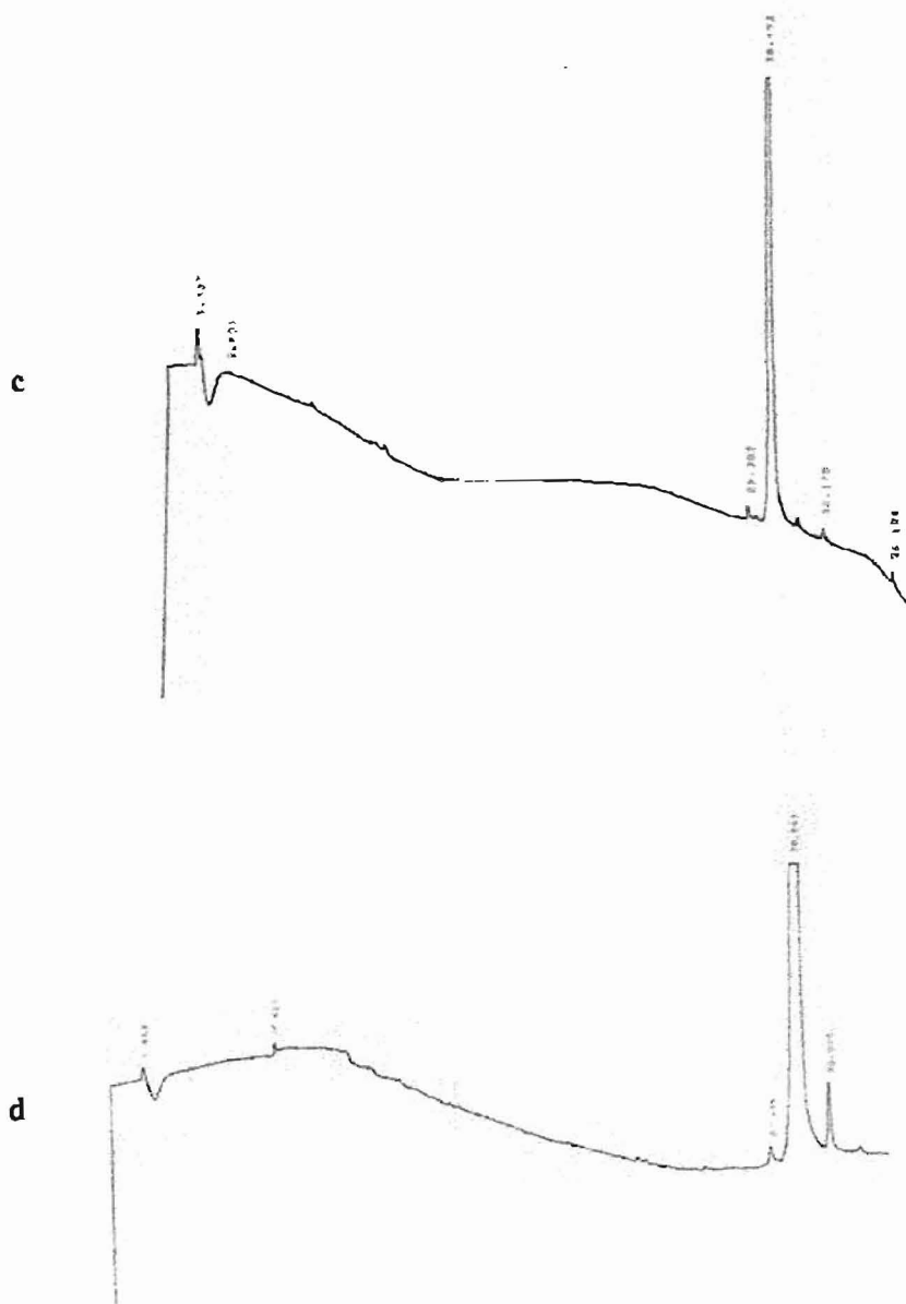
Figure 10: Analytical HPLC traces of purified oligonucleotides. Absorbance (260nm) vs. time (min) for (c) strand 3 and (d) strand 4. Both traces were obtained using linear gradient of NaCl (Table 1a)
